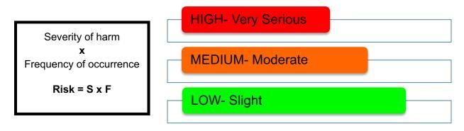
Determine the risk by combining Frequency (Probability) and Severity for each scenario. The highest severity found, is the level of risk associated with the job task.
